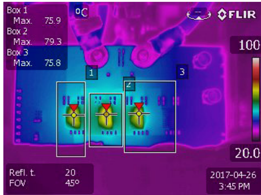
Figure 4. Thermal Capture at 12V IN , 1.0V OUT , 75A ( T_A = 25^{\circ}\text{C} , 200LFM Airflow and No Heat Sink)
